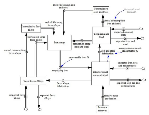
Figure 4 Iron supply chain presented by a System Dynamics Model (MinPol database 2017).
